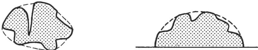
Figure 2.10 Irregularly shaped crack, and estimation method for effective area.
