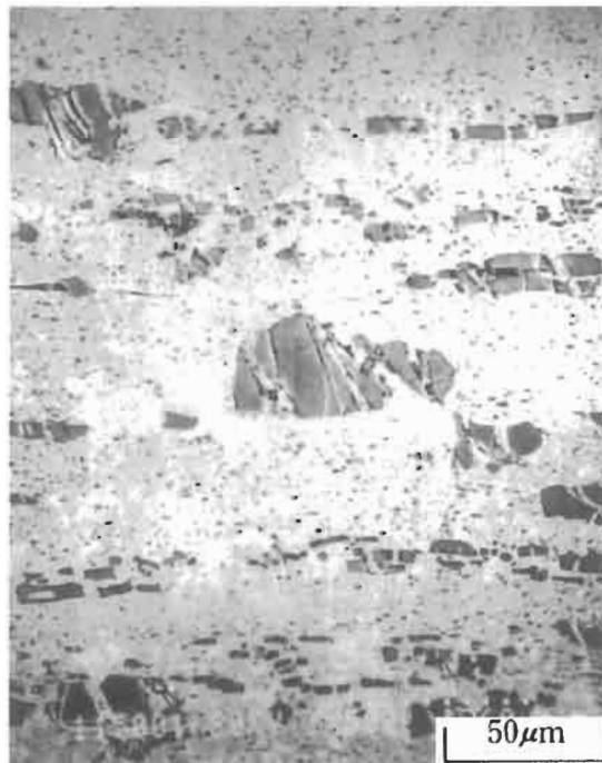
Figure 9.3 Microstructure of SKD-11 tool steel after heat treatment (Natsume et al. [4]).
